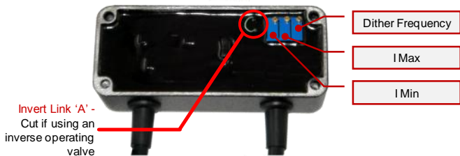
View of HFS 4 with lid removed and no cable shown for clarity
